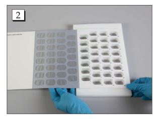
**Step 2.** Align the holes in the front of the card with the holes in the filling tray.
