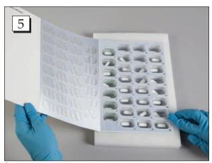
**Step 5.** Fold the card backing over, bringing it into position to seal the blister tray.
