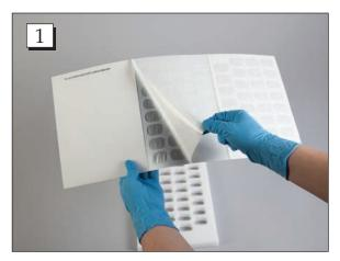
**Step 1.** Peel the paper backing from the card exposing the adhesive.
